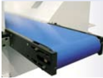
Chip conveyor integrated in the machine frame for disposing of the chips and waste parts
